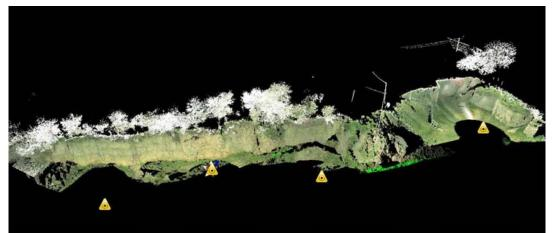
Figure 6 – Positions for individual clouds of points taken during 3D scanning at Vinča
