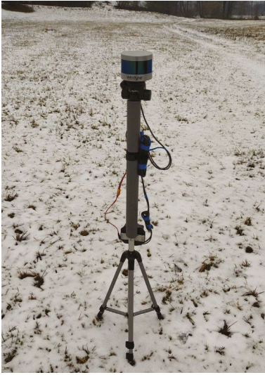
Figure 7. The first method of mounting the LiDAR Velodyne VLP-16 , used during archaeological prospection of the route of the highway Koridor Vc on the subsection Putnikovo Brdo-Medakovo near Tešanj.
