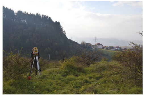
Figure 6. Topcon IS 9 Total station used during preliminary research at the Debelo Brdo site.
