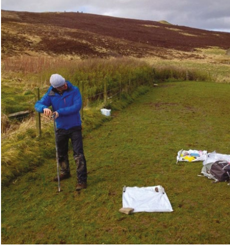
Figure 1. Using a Dutch hand auger on Mainland, Orkney, surveying midden deposits at a Neolithic settlement (photo: I. Ostericher)
