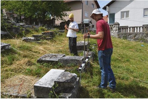
Figure 3. Geoscan Resistance Meter RM85 used during the geophysical survey of the Jewish cemetery in Sarajevo with modified spikes to enable recording between individual tombstones.
