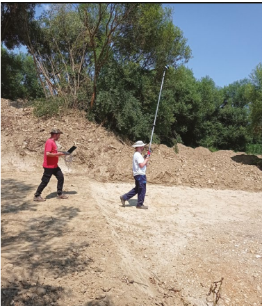
Figure 8. The second method of mounting the LiDAR Velodyne VLP-16 , used during the second research at the Nević Polje site, Lašva near Travnik.
