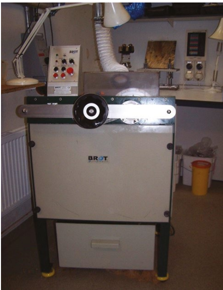
Figure 15. The Brot and its working area with the grinding wheel (left) and slide holder (right) (photo: T. Rajkovača)
