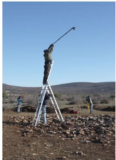
Figure 2. Photogrammetric single image technique workflow. Pod, near Bruška, 2011. (Photograph by Dinko Tresić Pavičić, courtesy of Kaducej d.o.o.)
