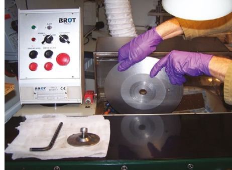
Figure 18. Changing the grinding wheel on the Brot machine (photo: T. Rajkovača)
