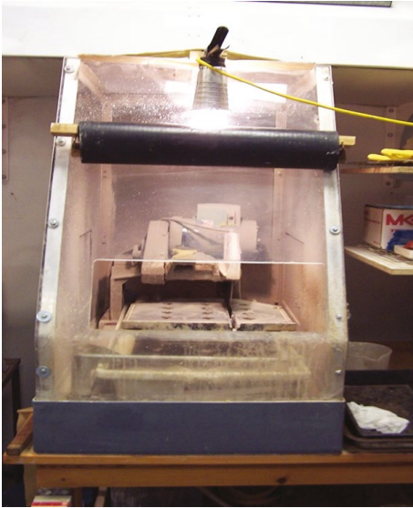
Figure 13. The diamond bladed saw for cutting slices (photo: T. Rajkovača)
