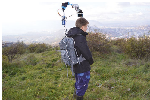
Figure 9. The third method of mounting the LiDAR Velodyne VLP-16 , used during preliminary research at the Debelo Brdo site.
