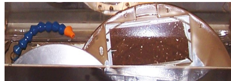
Figure 16. Sequence of beginning grinding after loading slides: 1: Turn the machine from hand to auto. 2: Turn on lubrication, and adjust the blue oil nozzle accordingly. Wind grinding wheel two turns away from the slides, against the arrow direction (Fig. 18). Set appropriate measurement to grind and set the gear. Close the machine's lid. 3: Start the grinding wheel. 4: Start the sample holder, and flick the gear on (photo: T. Rajkovača)
