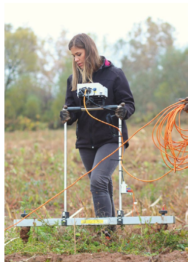
Figure 2. Geoscan Resistance Meter RM85 used during research at the Butmir site.
