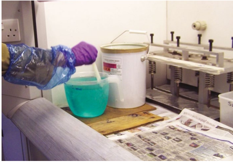
Figure 8. Impregnation with a mix of crystic resin, acetone, and MEKP accelerator/hardener (photo: T. Rajkovača)
