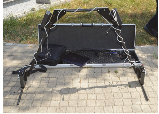
Figure 5. EasyRad Ground Penetrating Radar (GPR) used during the geophysical survey of a graveyard in Ljubuški.
