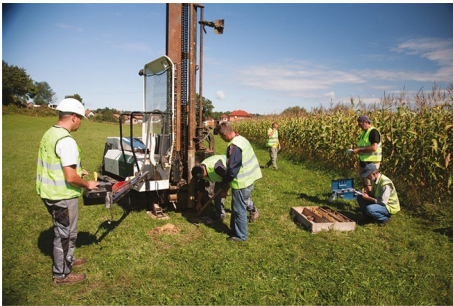
Figure 2. Using a machine corer for sampling a palaeochannel of the River Sana near Prijedor, Bosnia and Herzegovina (photo: I. Ostericher)
