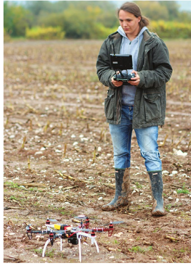
Figure 1. DJI Flamewheel F550 used during the research at the Butmir site with a student holding Flamewheel's remote control and a display that transmits visual information to facilitate the navigation of the UAV.
