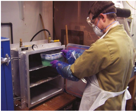
Figure 10. Placing impregnated samples in the vacuum chamber for 24-48 hours (photo: T. Rajkovača)
