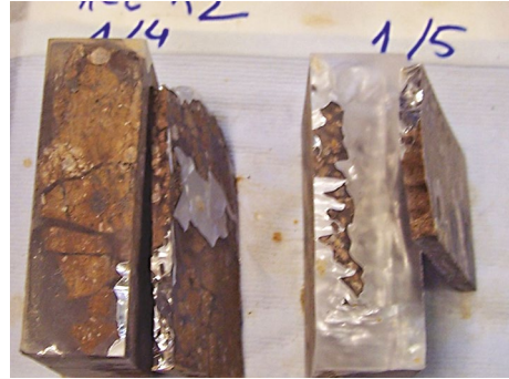
Figure 14. Cut blocks and slices cut with a notch to indicate the top of each sample (photo: T. Rajkovača)
