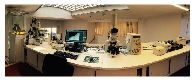
Figure 24: Equipment at LTFAPA Laboratory, Sapienza University of Rome. From left to right: Stereomicroscope, Metallographic microscope with transmitted and reflected light equipped with DIC and Confocal System, ultrasonic tank. (photo: <u>https://www.ltfapa.it/</u>)
