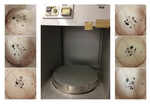
Figure 96: Experimental oven at LTFAPA (Sapienza University of Rome) and six phases of heating – the position of the tools inside the oven (photo A. Petrović)
